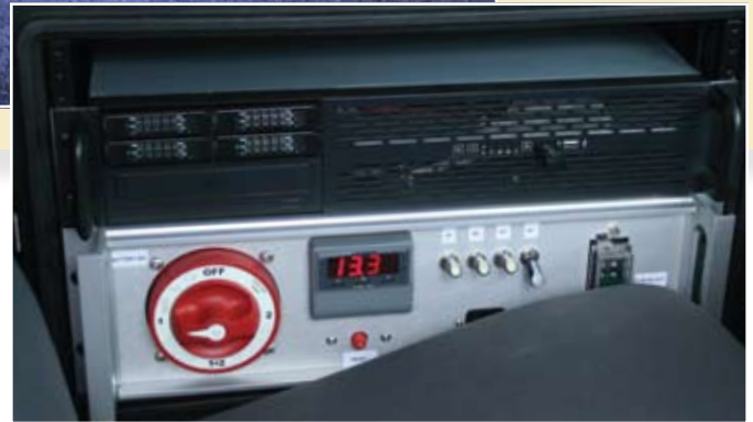
Below: Part of the IP-S2HD package, the data storage computer has an integrated power regulator and three removable 300 GB solid-state hard drives that allow easy data transfer to an office.
