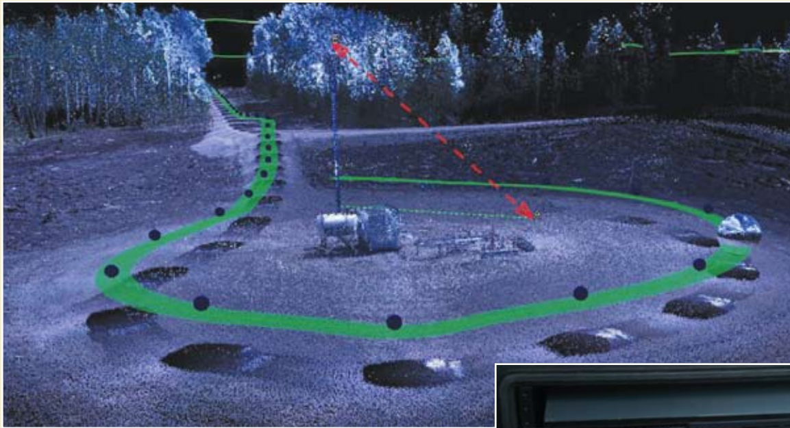
Left: Using Spatial Factory software, Vieworx can access the hidden point cloud behind the imagery, allowing for fast, accurate client asset inventory.
