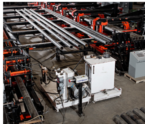
Structural Pipe/HSS Bundle Station
