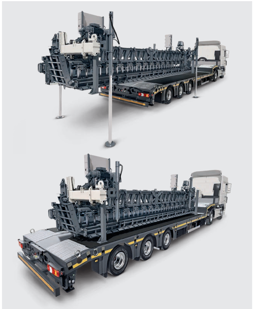
Self-loading dowel bar inserter.
