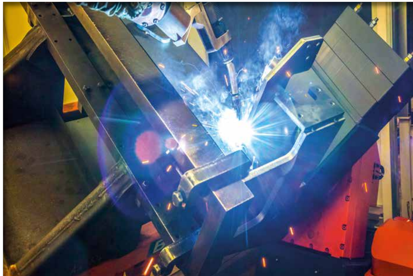
Welding cell for screed frames. Robot-produced weld seams feature consistent, high quality and precision.
