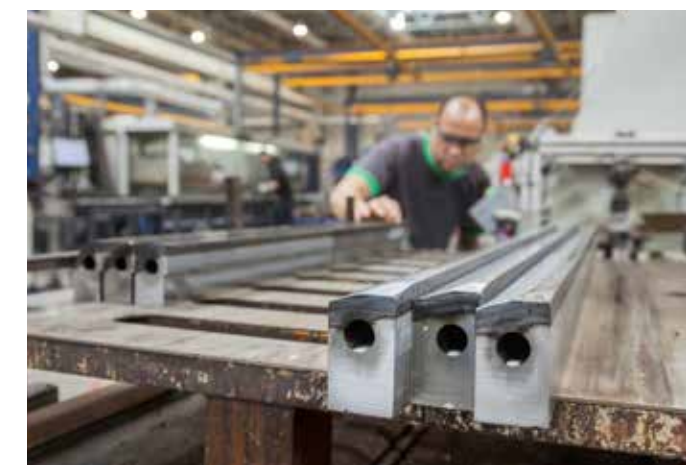
Tamper bar and pressure bar(s) are hardened to a uniform depth of 0.2 in (5 mm).
