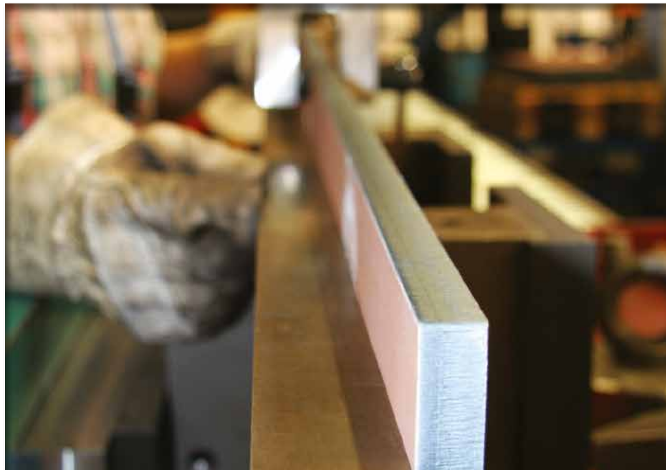
Screenshot plates straightened free from tension and with highest precision (error of no more than 0.008 in (0.2 mm) allowed) feature longevity thanks to even wear.
