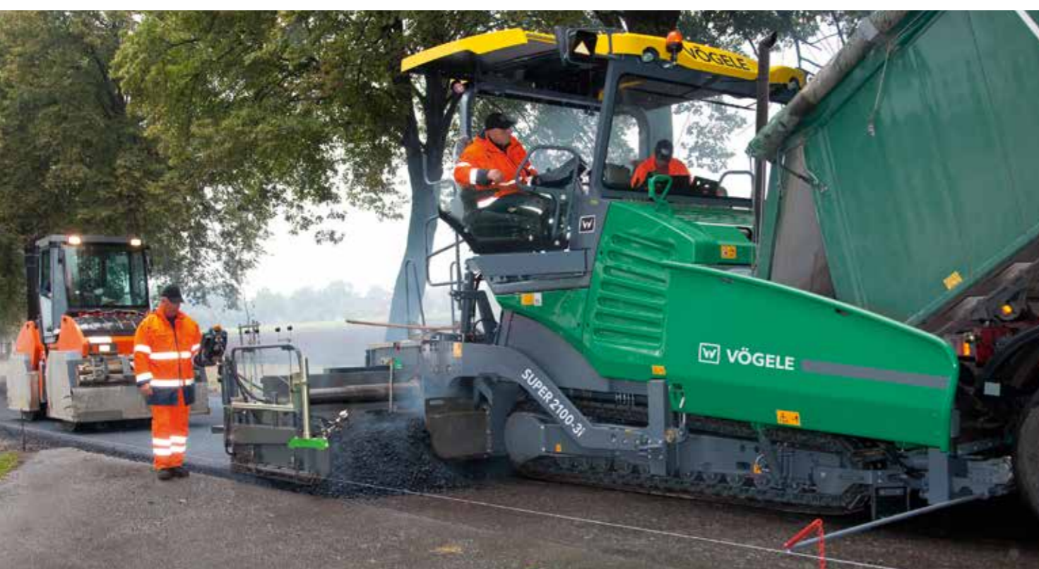
The power unit of the SUPER 2100-3i with its diesel particulate filter (DPF), diesel oxidation catalyst (DOC) and selective catalytic reduction (SCR) for exhaust gas after-treatment complies with the strict requirements of European exhaust emissions standard Stage V and US EPA standard Tier 4f.
