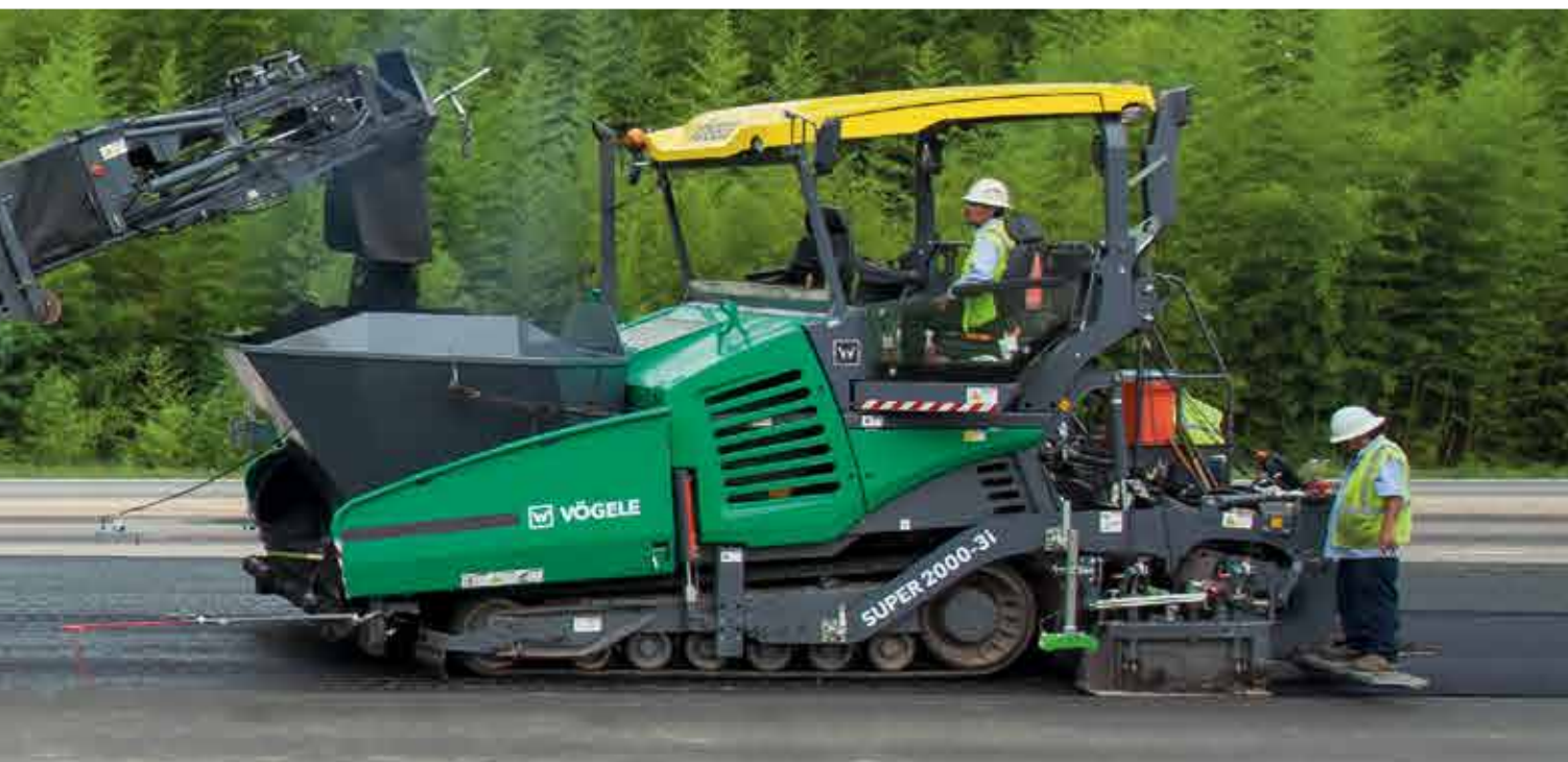
The power unit of the SUPER 2000-3i with diesel oxidation catalyst (DOC) and selective catalytic reduction (SCR) for exhaust gas after-treatment complies with the strict requirements of European exhaust emissions standard Stage 4 and US EPA standard Tier 4f.
