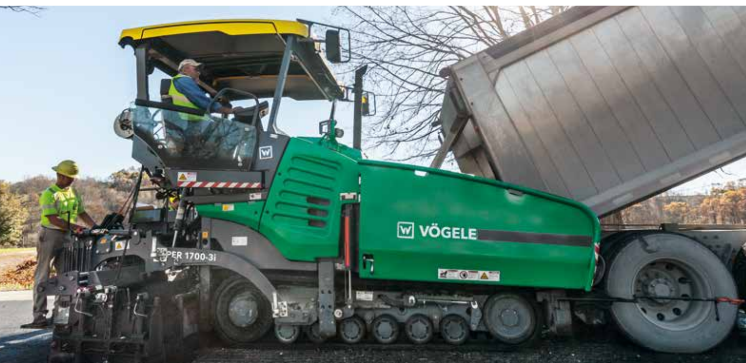
The power unit of the SUPER 1700-3i with diesel oxidation catalyst (DOC) and selective catalytic reduction (SCR) for exhaust gas after-treatment complies with the strict requirements of European exhaust emissions standard Stage 4 and US EPA standard Tier 4f.
