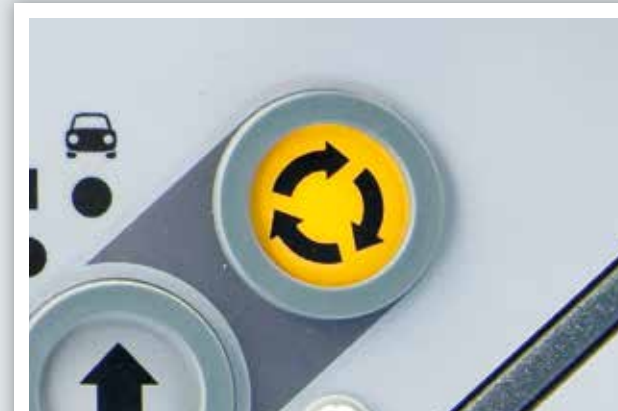
THE AUTOSET BASIC REPOSITIONING FUNCTION IS ACTIVATED JUST BY PUSHING THE "EXECUTE" BUTTON
